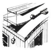
As shown in this diagram, when the COMMERCIAL 84 is applied on the area covered with Styrofoam, you get an all-proof tightness.
